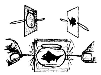
A thaumatrope is a toy device for demonstrating 'retinal retention.' This is the ability of the eye's retina to retain an image for a split second after the source of the image is withdrawn. A thaumatrope can be made as follows:
