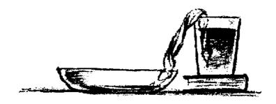
Dip a woman's handkerchief in water and wring it out. Then twist it like a rope, and hang it over the brims of two glasses arranged as shown. Be sure that the handkerchief touches the bottom of the higher glass, but hangs only a short distance below the rim of the lower one. Fill the top glass with water, and go away. By the next morning, you should find all the water in the lower glass.
