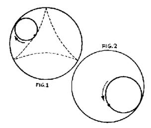
A hypocycloid is a curve traced by a point on the rim of a circle when the circle is rolled around the inside rim of a larger circle. For example, Fig. 1 shows a three-cusped hypocycloid, called the 'deltoid,' that results when the rolling circle has a diameter one-third that of the larger circle.
