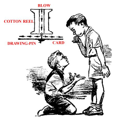
Push a drawing pin through the centre of a playing card and place a cotton reel over the point of the pin as shown. Holding the cotton reel in one hand and the card in the other, put your lips to the top and blow down through it as hard as you can. At the same time, release the card.
