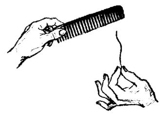
The famous Hindu rope trick may be a myth, but here is a miniature version of it that anyone can do. Hold one end of a short piece of thread. With your other hand, rub a pocket comb briskly on your clothing, and then bring it near the free end of the thread. You will find you can make the thread stand upright as shown. If you move the comb in small circles, the thread will also move in small circles.
