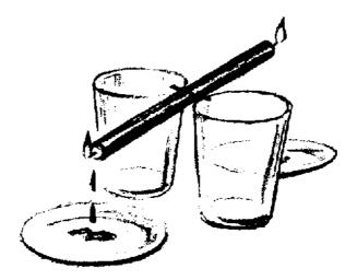
A perpetual-motion machine operated solely by gravity is impossible, but gravity does play an essential role in thousands of simple mechanical devices. Here is a gravity machine you can construct from a candle, a needle, two glasses, and two saucers.
