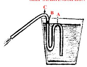
Many strange types of self-starting siphons have been invented, but this one is so elementary that you can construct it yourself from a single piece of glass tubing.
