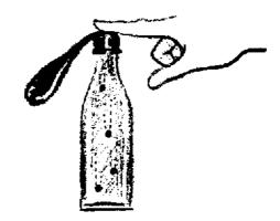
Pascal's law tells us that pressure applied to a confined liquid is transmitted undiminished to all parts of the liquid. This can be demonstrated with an empty bottle, a few paper book matches, and a balloon.
