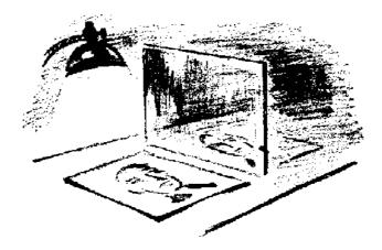
We are familiar with the fact that a windowpane will reflect images like a mirror, especially at night when the far side of the window is dark and the room is illuminated. This fact can be put to practical use in making an excellent device for copying drawings.
