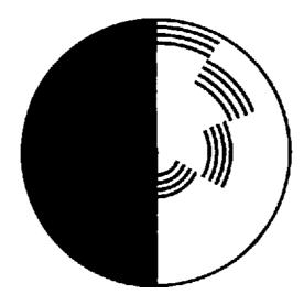
'Subjective colour' is the term physicists apply to colours that appear when you are watching rapidly alternating patterns of black and white. To demonstrate this puzzling phenomenon, copy the circle shown and mount it on cardboard. Push a pin through the centre dot so you can spin the disc.
