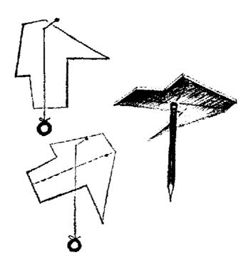
The centre of gravity of an irregularly shaped piece of cardboard is the spot where it will balance on the eraser of a pencil. Here is an interesting way to locate this spot.
