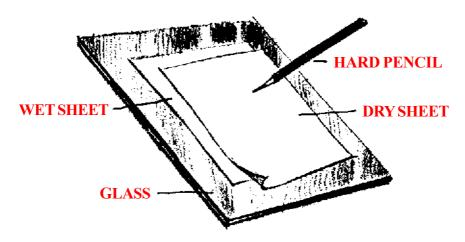
As every stamp collector knows, a watermark is an invisible imprint on a postage stamp, for identification purposes. It becomes visible when the stamp is immersed in liquid. Applying pressure that disturbs the fibres of the paper produces watermarks and thus changes the way they reflect light when wet. Watermarks are easy to make and provide a novel, little-known way to write secret messages.
