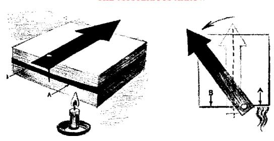
Unlike most substances, rubber contracts when heated, expands when cooled. This can be demonstrated by the following experiment.
