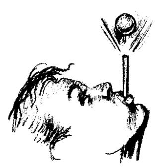
Cut a six-inch piece from the end of a straw. Put one end of the piece on your mouth, tip back your head, and hold a table-tennis ball a few inches above the other end. Blow as hard as you can, simultaneously releasing the ball. Instead of being blown away as you might expect, it remains suspended in mid-air. The harder you blow, the higher it floats above the straw.
