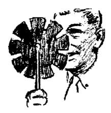
A stroboscope is a device that cuts off light at regular intervals of time. When you look through it at a rhythmically moving object, the motion seems to slow down or even to stop. A simple stroboscope is easily made by cutting eight narrow slots at evenly spaced intervals around the rim of a cardboard circle. Put a pin through the centre, and stick the pin into the eraser of a pencil so you can spin the disc in front of one eye, as shown.
