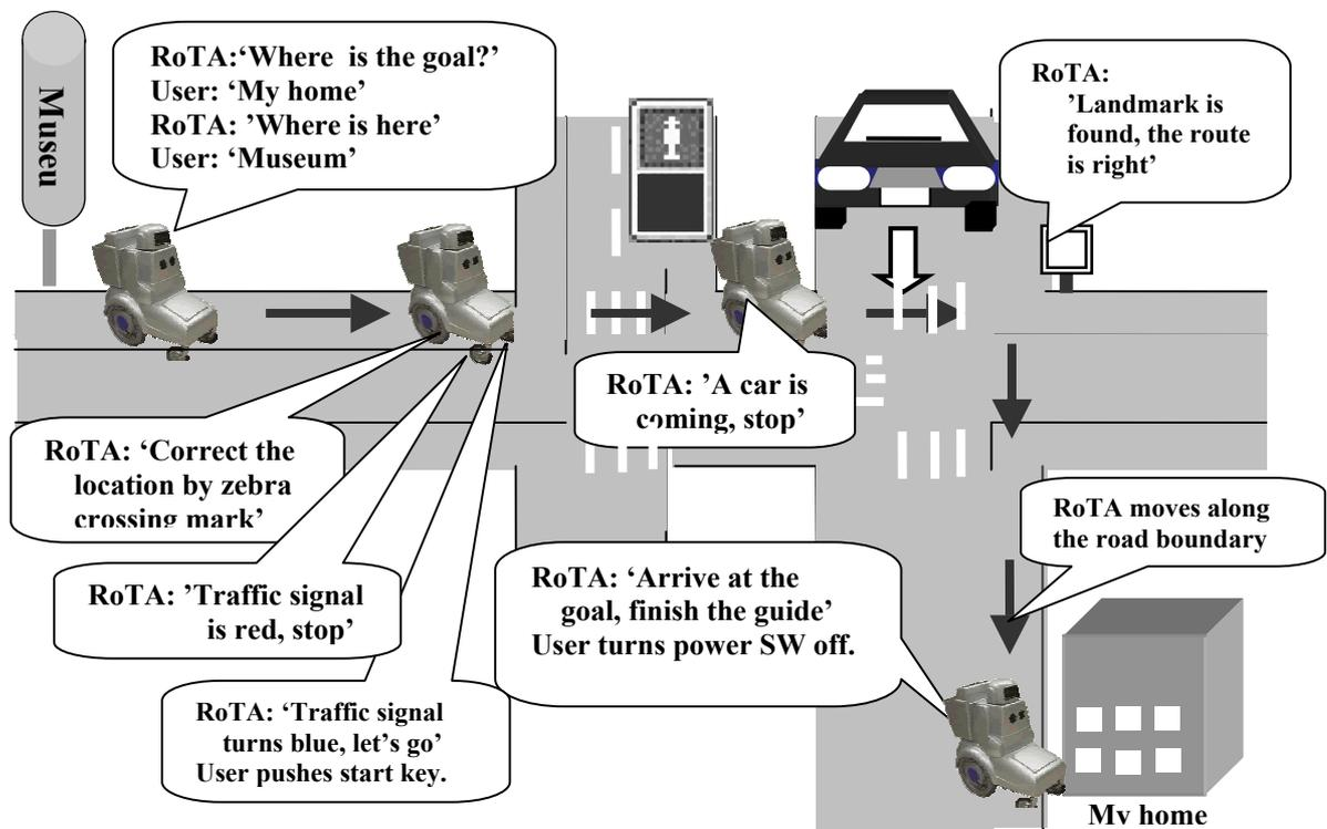
Figure 10. An illustration of the RoTA guide.
