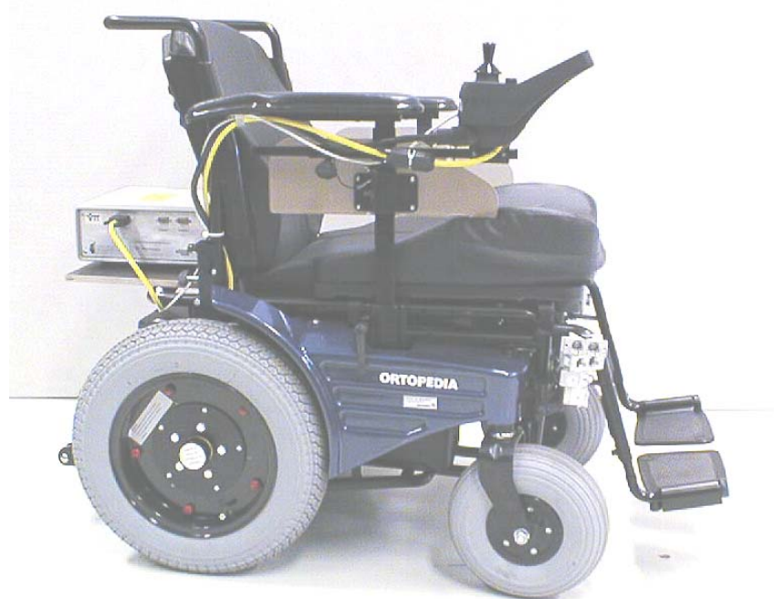
Figure 3. Here the obstacle avoidance unit is attached to a standard electric wheelchair. Notice the ultrasonic sensors in the front, and the electronic obstacle avoidance unit at the back. The rear sensors can not be seen from this angle.
